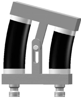
图 2 侧摆关节的运动状态示意图 Fig.2 Bending state of side-sway joint
