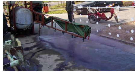
图6 防飘性能试验现场 Fig.6 Anti-drift performance test
