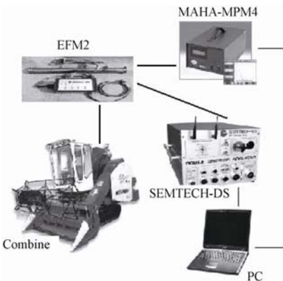
注: Combine 为测试的联合收割机; PC 为笔记本电脑; SEMTECH-DS、EFM2 和 MAHA MPM-4 分别是机动车尾气排放气态污染物分析仪、尾气质量流量计和尾气排放颗粒物的测试仪。 Note: Combine stands for the tested combines, PC is a personal computer, SEMTECH-DS is used to test instantaneous exhaust gaseous emissions from vehicle; EFM2 is used to measure instantaneous exhaust mass flow rates from the vehicles; MAHA MPM-4 is used to measure particle mass.
