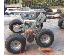
b. 人形腿后轮越障试验 b. Test of second humanoid wheel obstacle-surmounting
