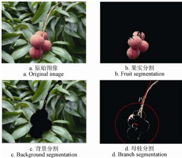
注: P 为采摘点; C_p 为果实图像区域的质心。 Note: Point P is picking point; point C_p is centroid location.
