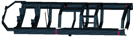
b. 船式拖拉机机架有限元模型 b. Finite element model of boat-type tractor rack
