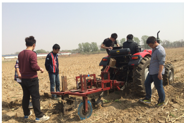
图 10 免耕播种机土壤工作部件测试装置的安装与调试 Fig.10 Installation and adjustment of soil working tool testing device of no-till planter
