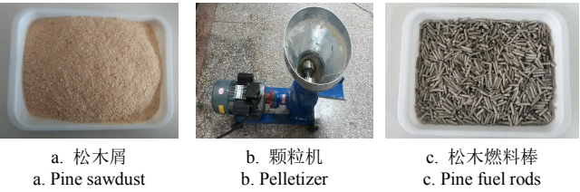
图 1 生物质气化原料与装备 Fig.1 Experimental materials and device for biomass gasification
