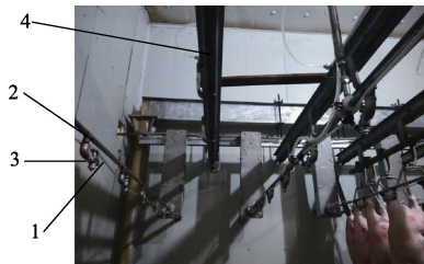
1. 气管 2. 水管 3. 喷嘴 4. 猪胴体悬挂轨道 1. Gas pipe 2. water pipe 3. Spray nozzle 4. Tracks for hanging pig carcasses
