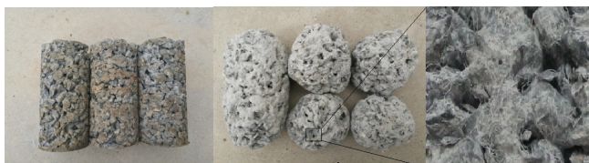
a. 试块冲击磨损前 a. Specimens before impact abrasion b. 试块冲击磨损后 b. Specimens after impact abrasion
