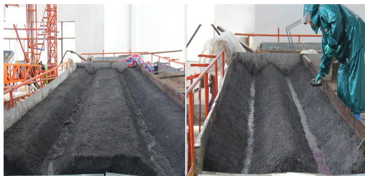
a. 顺坡宽垄 a. Wide longitudinal ridge tillage b. 顺坡窄垄 b. Narrow longitudinal ridge tillage
