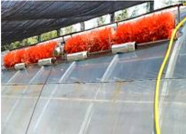
图7 样机清洗试验 Fig.7 Cleaning test of prototype
