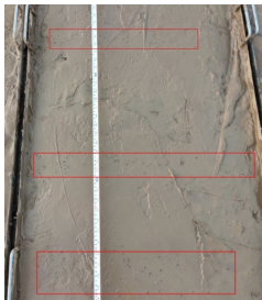
图 12 泥盒中油菜种子籽粒典型分布状况(导种装置高度 2 m) Fig.12 Typical distribution of rapeseeds in the mud box (height of seed guiding device is 2 m)
