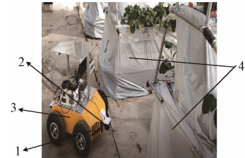
1.车底盘遮挡区域 2.前激光雷达 3.车载系统 4.草莓架 1.Vehicle chassis shelter area 2.Front lidar 3.On-board system 4.Strawberry shelf
