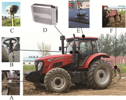
图 1 拖拉机自主行驶与作业机组组成 Fig.1 Composition of autonomous driving and working unit for tractor
