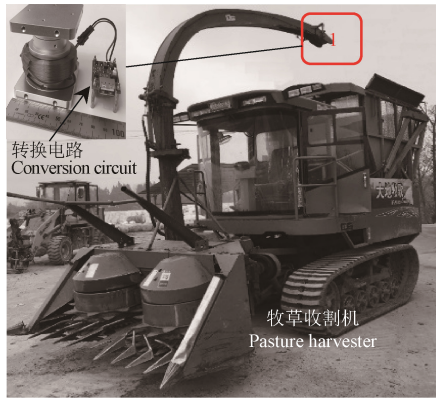
图 9 俘能器应用 Fig.9 Application of the energy harvester
