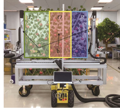
a. 机械臂 b. 深度相机 c. 嵌入式计算机 L. 左机械臂专属作业区域 R. 右机械臂专属作业区域 O. 重叠作业区域 a. Mechanical arm b. Depth camera c. Embedded computer L. Exclusive operating zone of left mechanical arm R. Exclusive operating zone of right mechanical arm O. Overlapped operating zone
