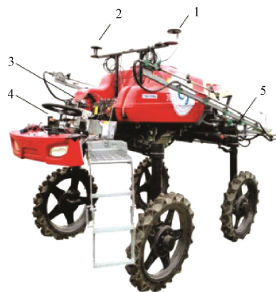
1.定位天线 2.定向天线 3.行走控制机构 4.转向电机 5.喷雾阀组 1.Positioning antenna 2.Vector antenna 3.Driving control mechanisms 4.Steering motor 5.Spraying valve group
