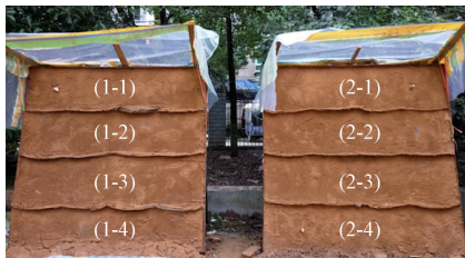
注: (1-1) 为 1 号喷灌边坡 1 号分区, (2-1) 为 2 号壤中滴灌边坡 1 号分区, 同理类推。其中, 各边坡的 1、3 号分区设有灌溉支管。 Note: (1-1) refers to No. 1 partition of No. 1 sprinkler-irrigation slope, (2-1) refers to No. 1 partition of No. 2 buried-drip-irrigation-in-soil slope, and so on. Among them, the No. 1 and No. 3 partitions of each slope are equipped with irrigation branch pipes.
