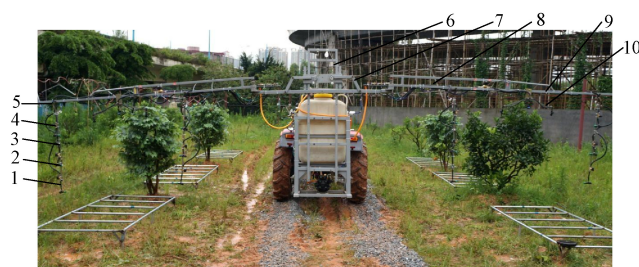
b. 试验现场 b. Testing field 1.喷雾软管 2.喷头 3.吊挂喷杆 4.电磁阀 5.双十字万向节 6.升降导轨 7.升降架 8.一级展臂 9.二级展臂 10.倒 Y 型喷头支架 1. Spray hose 2. Nozzle 3. Hanging spray bar 4. Solenoid valve 5. Double cross universal joints 6. Lifting guide rail 7. Lifting frame 8. Primary boom 9. Secondary boom 10. Inverted Y-type nozzle bracket
