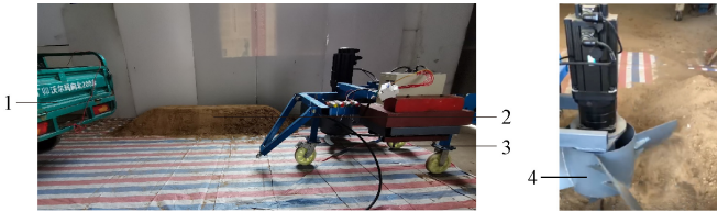
1.电动车 2.试验土垄 3.试验台架车 4.旋抛刀具 1.Electric vehicle 2.Test soil ridge 3.Test bench 4.Rotary throwing cutter
