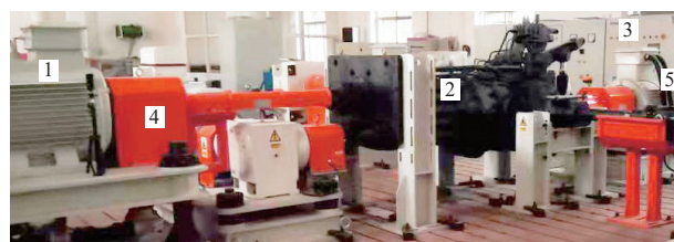
1.驱动电机 2.HMT 装置 3.测控系统 4.转速转矩仪 5.加载电机 1. Driving motor 2. HMT device 3. Measurement and control system 4. Speed/torque sensor 5. Loading motor
