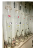
c. 蒸渗仪地下水供排水装置 c. Groundwater supply and drainage device for lysimeter
