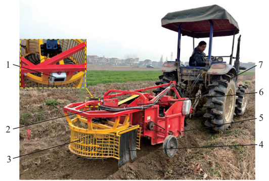
1. 霍尔传感器电子数显表 2. 液压马达 3. 离心圆盘式根土分离装置 4. 侧向抛送橡胶帘 5. 振动挖掘铲 6. 栅条式筛分装置 7. 三点悬挂机构 1. Hall sensor electronic digital display 2. Hydraulic motor 3. Centrifugal disc type root and soil separation device 4. Lateral throwing rubber curtain 5. Vibrating excavation shovel 6. Grating type screening device 7. Three point suspension mechanism
