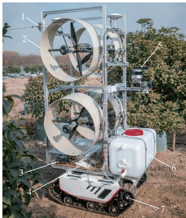
1. 差分信号接受天线 2. 风送式喷雾结构 3. 导航处理器 4. AI 边缘计算机 5. 双目相机 6. 水箱 7. 差速履带底盘 1. Differential signal receiving antenna 2. Air-assisted spray structure 3. Navigation processor 4. AI edge computing device 5. Binocular camera 6. Water tank 7. Differential track chassis
