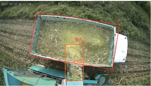
图 11 物料及车厢的实时检测 Fig.11 Real time detection of materials and carriage
