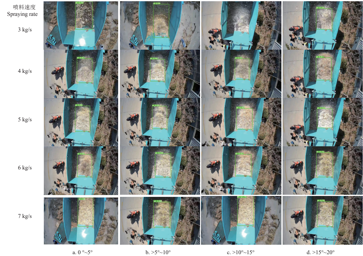
图 10 不同喷料速度及喷料角度下物料检测结果 Fig.10 Material testing results at different spraying speeds and spraying angles
